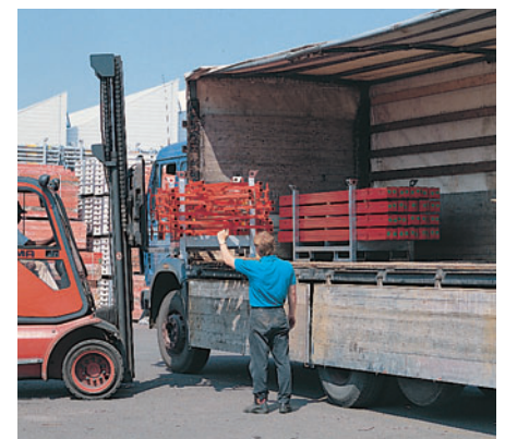
PERI post pallets can be shifted easily with a fork-lift truck.
